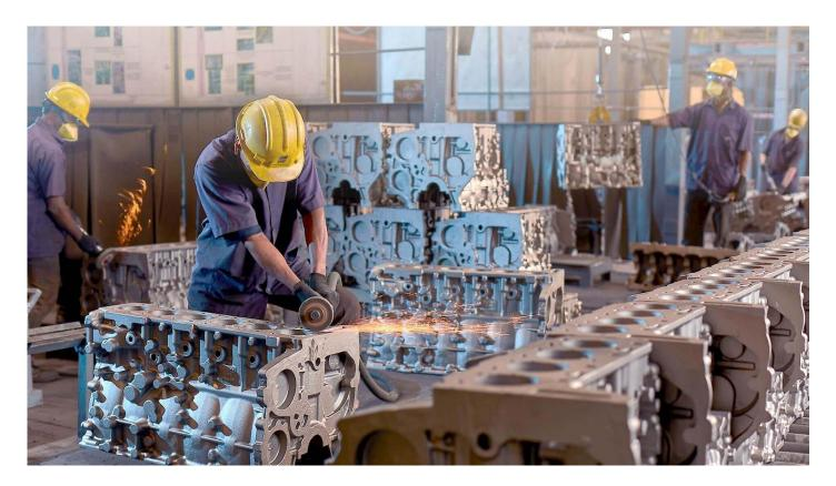
Our cylinder block, head castings and housing are used in a wide range of engines, across construction machines, farm equipment and utility vehicles made by some of the world's largest automobile
